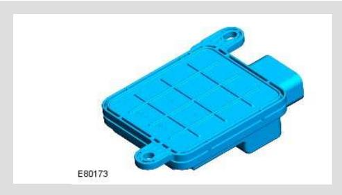
The occupancy sensor module is installed on the underside of the front passenger seat. The module supplies a power feed to the occupancy sensor and monitors the return voltage to determine if the seat is occupied or not. The result is transmitted to the RCM on the High speed CAN bus. The occupancy sensor module also monitors for short and open
