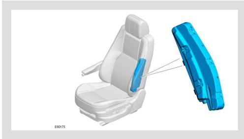
A side air bag is attached to the outside of each front seat backrest frame, under the backrest cover.
