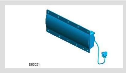
The inflatable knee bolster air bag is located behind the driver's knee bolster panel below the steering column. The flanges of the inflatable knee bolster air bag are attached to a re-enforcement lid in the driver knee bolster panel. The re-enforcement lid incorporates two deployment doors that are forced open, splitting the instrument panel covering, when the air bag deploys.
