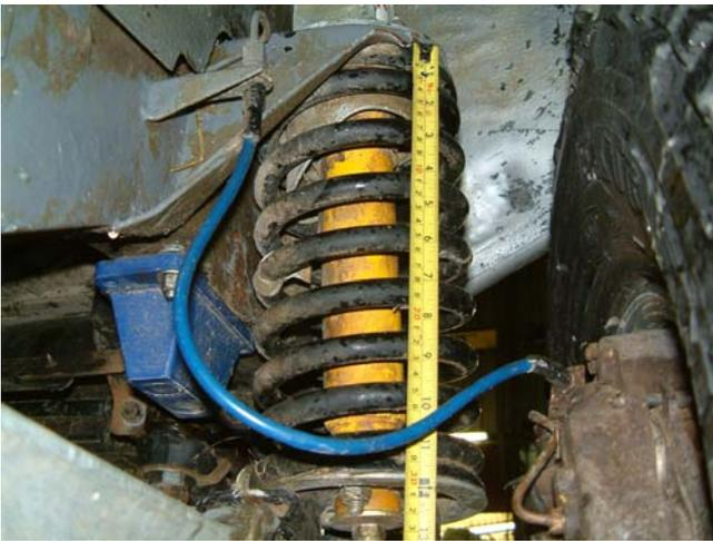
You need to measure the rear part of the front coil spring from where it touches the chassis down to where it touches the spring seat.
