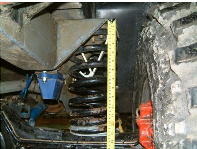
You need to measure the rear part of the rear coil spring from where it touches the chassis down to where it touches the spring seat.
