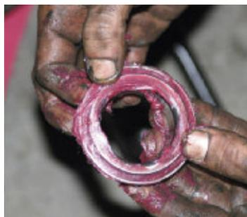
Fig 11 - Repacked bearing ready to install into hub.
