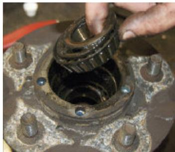
Fig 6 - Removing outer bearing.
