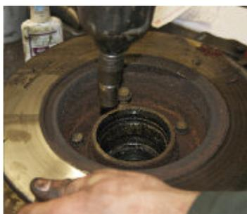
Fig 8 - Removing hub bolts.
