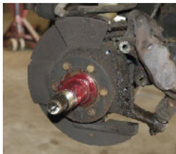
Fig 16, 17 - Grease stub axle before putting hub-disc back into place. Remember to hold caliper to side when fitting hub-disc assembly. With the caliper in hand, get a feel for the tension of the brake lines. Be very careful to not put stress on the brake lines.
