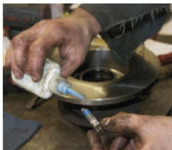
Fig 13 - Coupling hub to disc.
