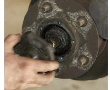
Fig 3 - Pulling drive member off with bolts removed.
