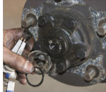
Fig 2 - Circlip, (2) driveshaft shims.
