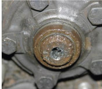
Fig 1 - Hub assembly with dust cover removed.
