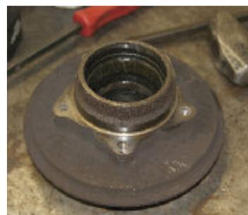
Fig 9 - Separated hub from disc.
