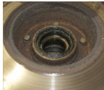
Fig 7 - Remove the grease seal and inner bearing.
