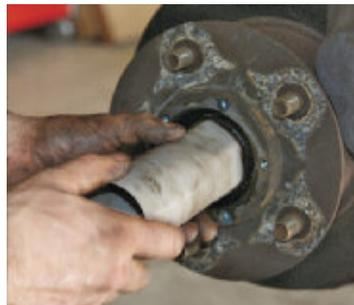
Using the hub nut removal tool RNF406.
