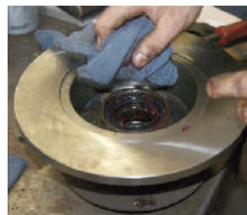
Fig 15 - Install inner bearing and new grease seal. Note: A round drift can be used to install the seal; be careful to not damage when installing.
