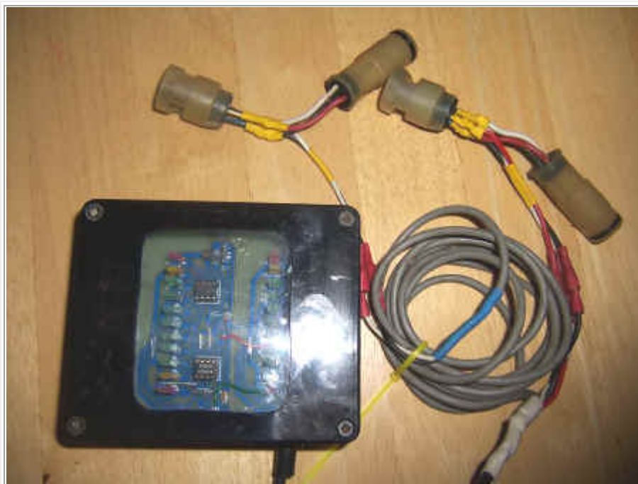
A simple test box that monitors both lambda outputs
