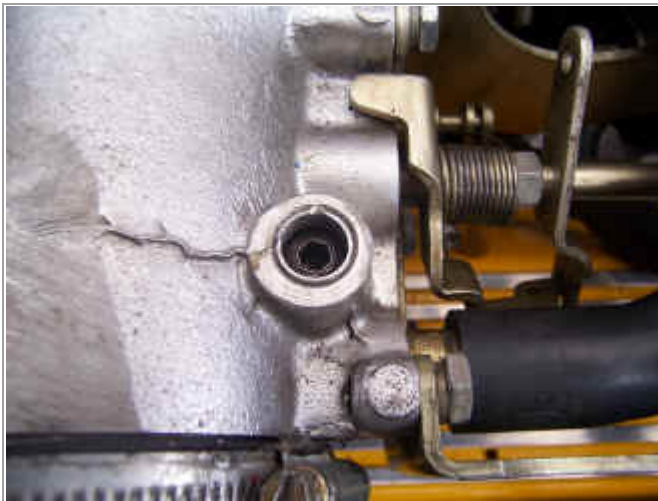
Base Idle adjustment screw.
