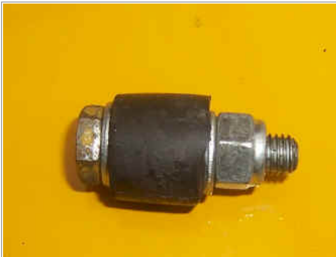
Make up a sealing plug with a M6 bolt and a bit of fuel hose. Tightening the bolt will expand the hose to provide a good seal (see below).
