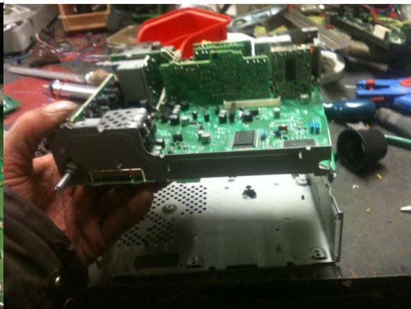
5. Next remove the aluminium heat sink, this has 3 screws that secure the regulators to it. And just lifts away. Below is a metal bracket that the heat sink screws go through to, its has twist tabs that are soldered to the board underneath, these will have to be desoldered and the part removed, again be careful as i believe this acts as a ground so dont damage the
