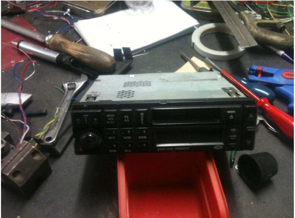
1. With the radio on the bench, remove the 4 screws and gently pry the top cover off, starting at one side and working your way around. Pictured below.
