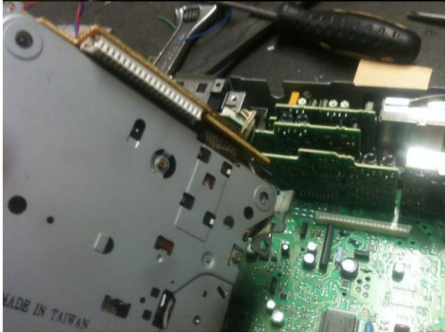
4. Next remove the 4 extension bolts that the tape deck was secured to, these are 6mm. Then on the main board there is a twist tab, turn this to align it with the slot, and cautiously lift the board from the main housing. Be very careful as if you have not aligned the tab correctly you could break the board. (studs marked in red, tab in blue)
