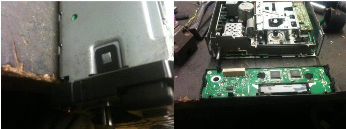
3. Next remove the tape unit, this is 4 screws, circled. As with the front panel, it is also on a multi plug, located at the rear of the tape deck, may take a little wiggling as is can be tight.
