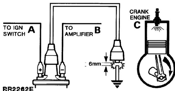
Remove coil/distributor H.T. lead from distributor cover and hold approximately 6mm from engine block, using suitable insulated pliers. Switch ignition 'On' and operate starter.
