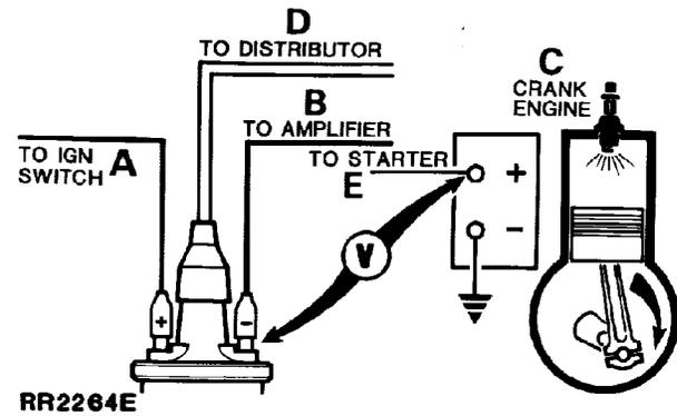
Connect voltmeter between battery positive (+ve) terminal and H.T. coil negative (-ve) terminal. Voltmeter should register 0 volts.
