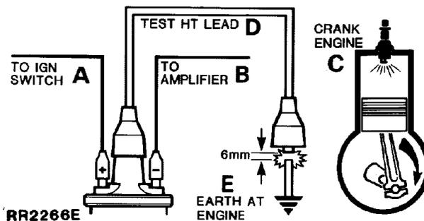
Remove existing coil/distributor H.T. lead and fit test H.T. lead to coil tower. Using suitable insulated pliers, hold free end about 6mm from engine block and crank engine. There should be good H.T. sparking.
