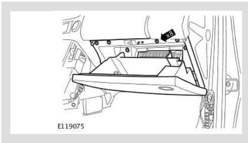
Remove the 8 screws from the lower glove compartment.
