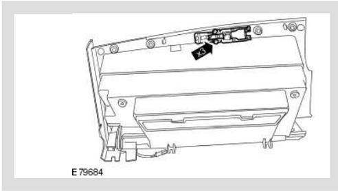
Remove the lower glove compartment latch.
