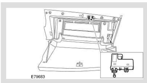
Remove the lower glove compartment lamp.
