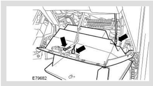
Remove the lower glove compartment.
