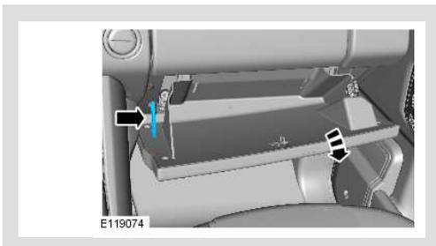
Open the lower glove compartment to the service position.
