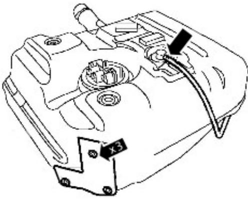
**11.** Remove the fuel tank vent line.
