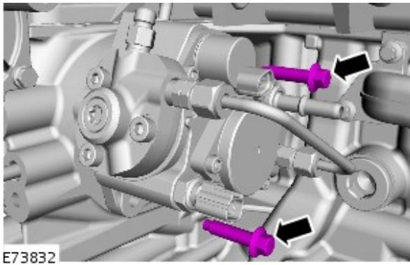
**18. Using the special tool, release the fuel injection pump.**
