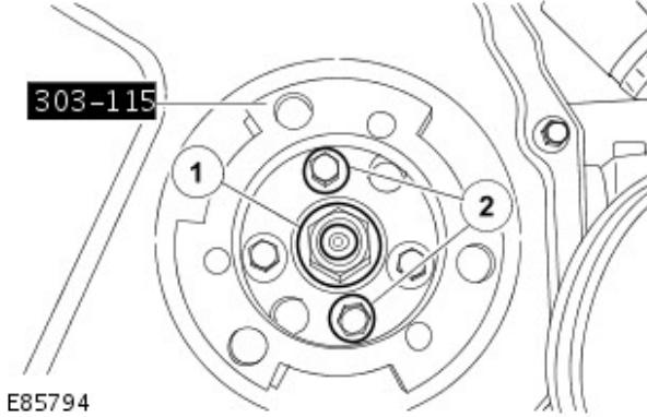
**17. Remove 2 bolts from the fuel injection pump.**
