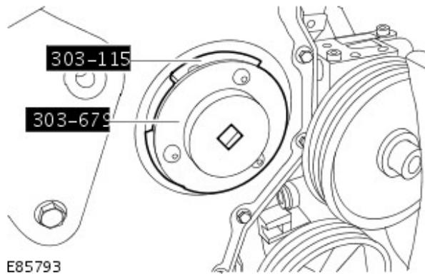
**16. Release the fuel injection pump drive gear.**
