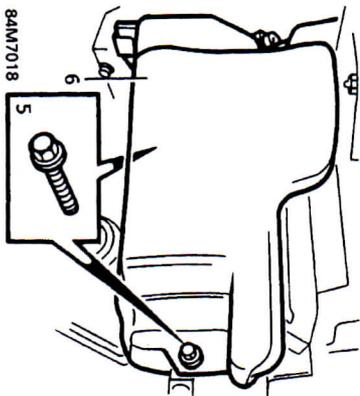
6. Release reservoir from mounting for access to washer pumps.
