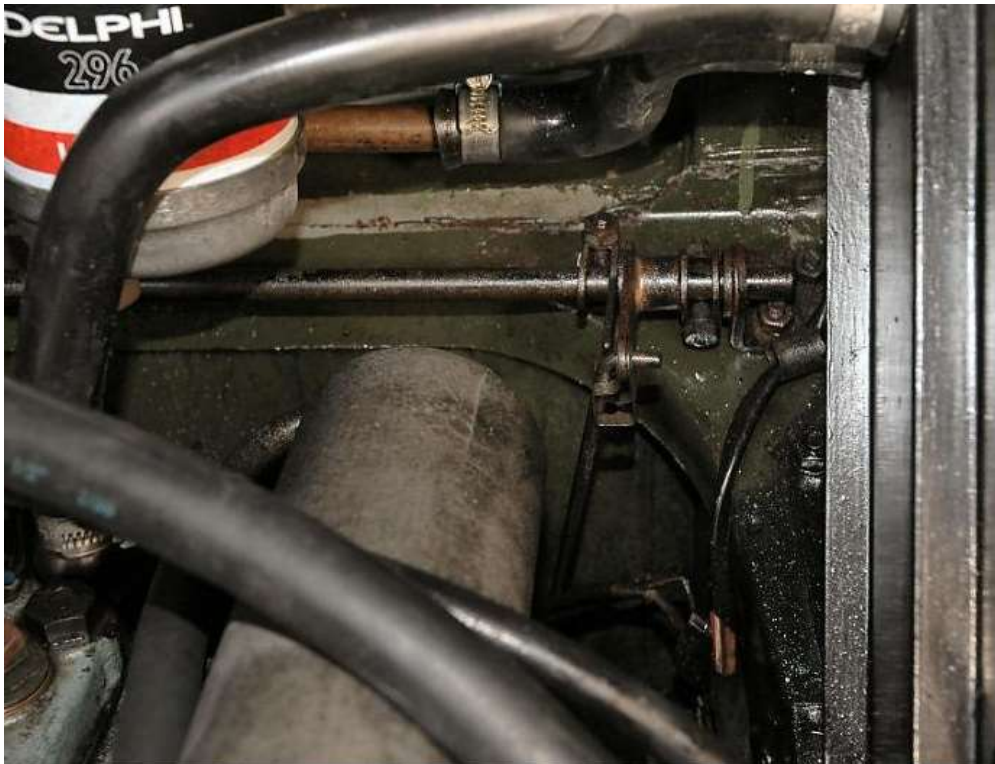
GROUP H ACCELERATOR - Engine Speed Hand Control 2 1/2 Litre Diesel
