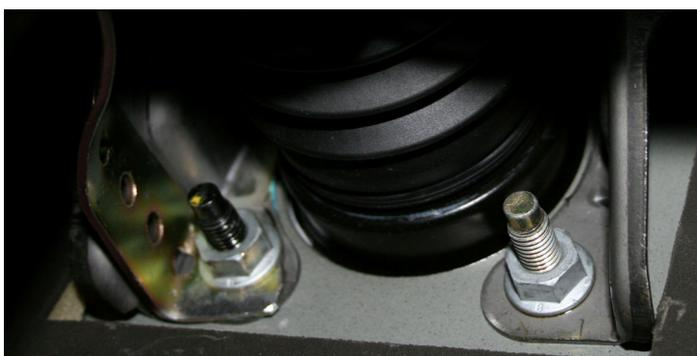
Above shows the reed switch and magnet positioning, this has the reed closed when the clutch is released (at rest) and the switch opens as soon as the pedal moves from rest (before the clutch bites). Check this with a meter or lamp and bend the bracket to adjust the switching point. This is to stop the engine over-revving when the clutch is used while CC is on – important safety over-ride for CC. Picture on the left is a clearer view of the bracket mounting.
