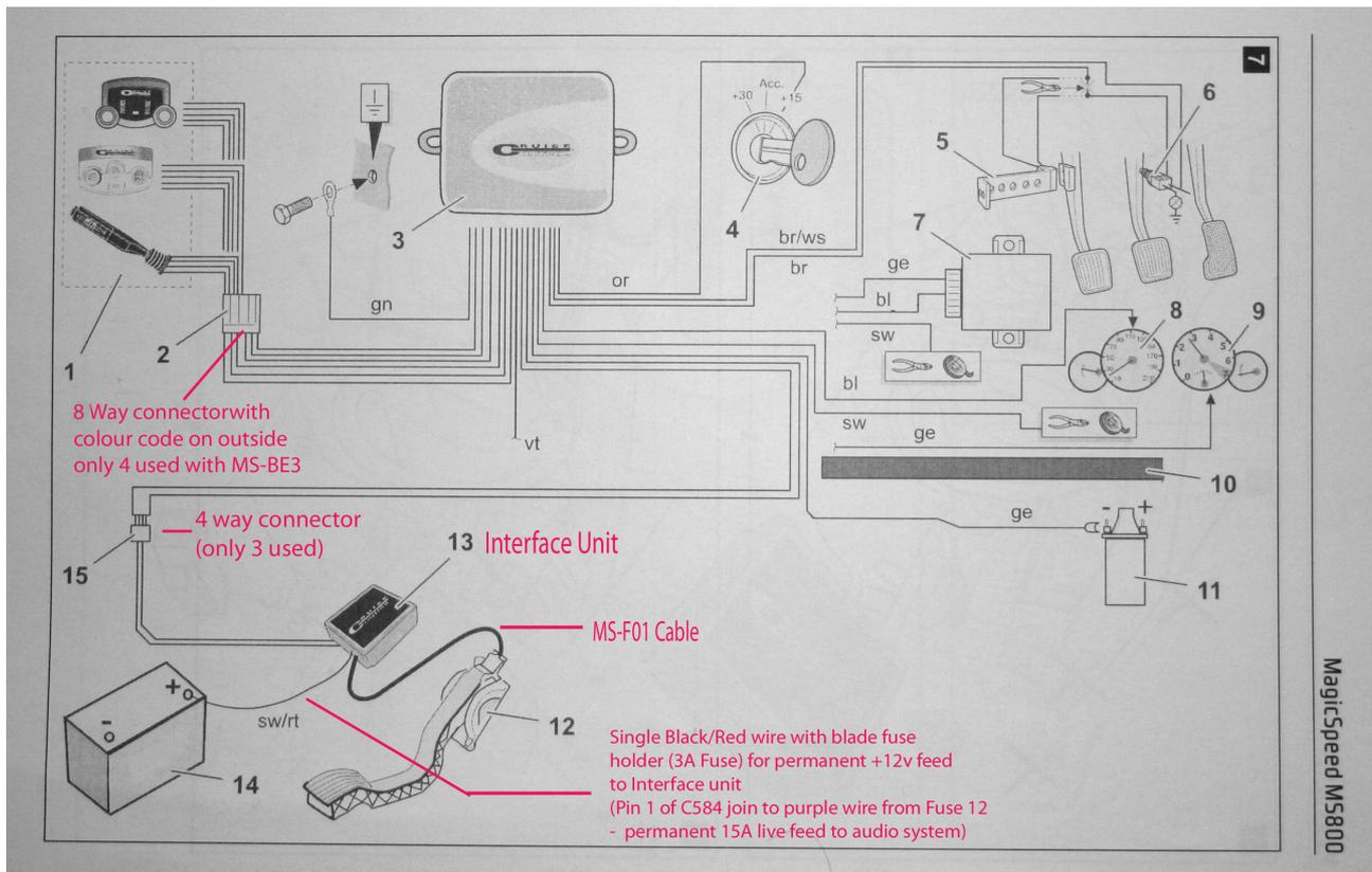
I checked out the various ways that the WACO unit can be connected up and decided that the simplest if not most elegant was the magnetic clutch switch and road speed input combination. The installation manual does cover all of the options available in several languages.
