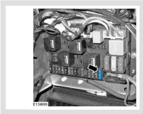
Remove fuse 16 (5 Amp) from the rear loadspace fuse box.
