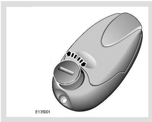
Remove and install the transmitter battery.
