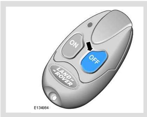
Install fuse 16 (5 Amp), and within 5 seconds press the OFF button on the transmitter for at least 1 second.
