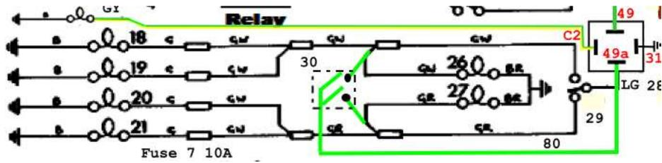
Double pole rocker switch to give hazard lights on a series.
