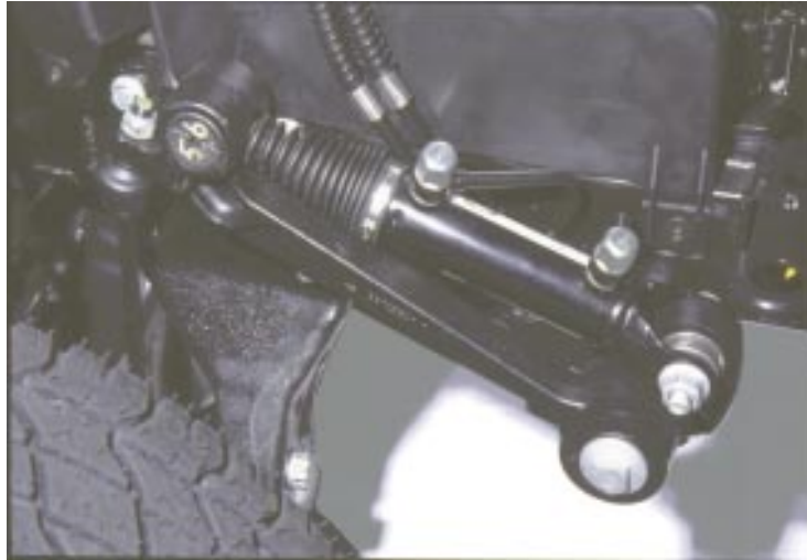
Figure 96 Front actuator
