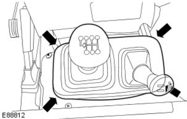
7. **⚠ WARNING:** The gearshift lever knob will be released suddenly, keep face clear during removal. Failure to follow this instruction may result in personal injury.
