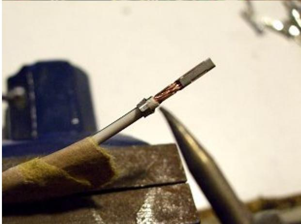
Not having ABS I cut a small length to bend round into the appropriate pins. Before pushing them into the plugs I double checked all the positions and snapped shut the plugs.
