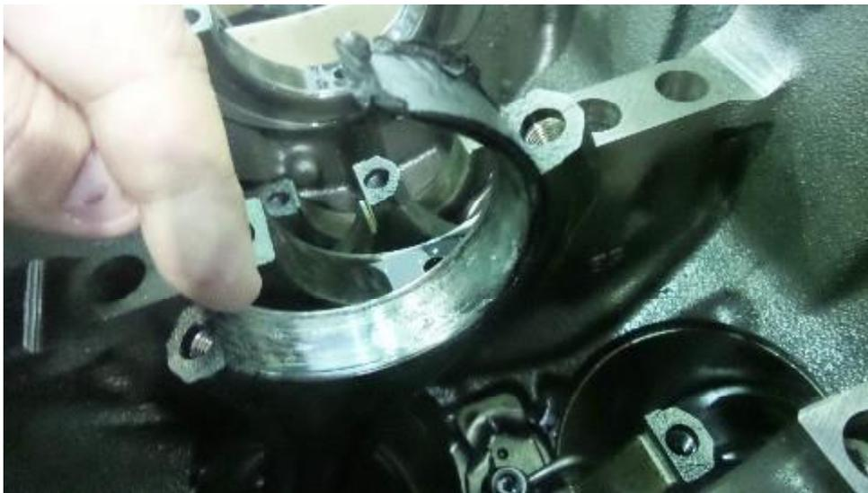
Fig. № 9. The connecting rod is welded by friction liner motor vehicle investigated LAND
