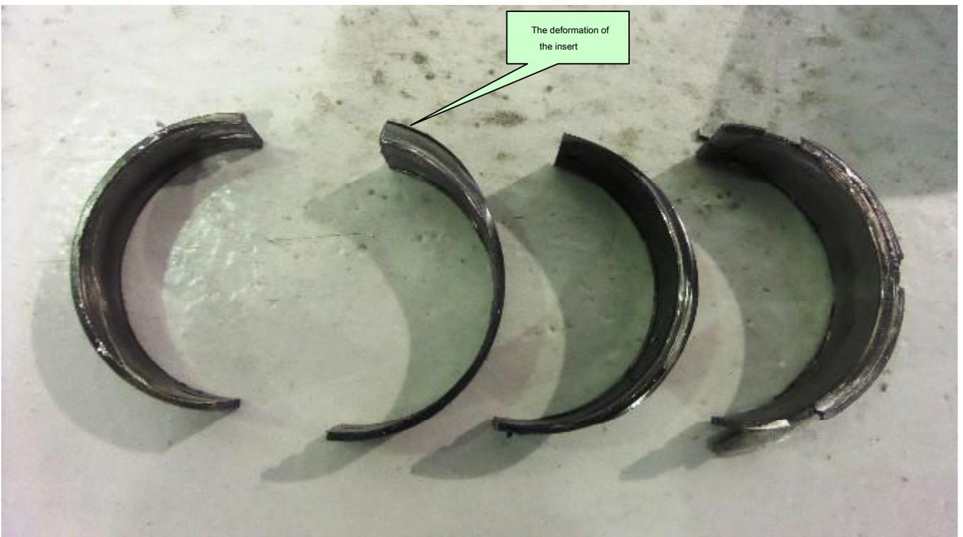
Fig. Number 14. Status of indigenous inserts after removing the crankshaft of the engine of the test vehicle LAND ROVER DISCOVERY 4,
