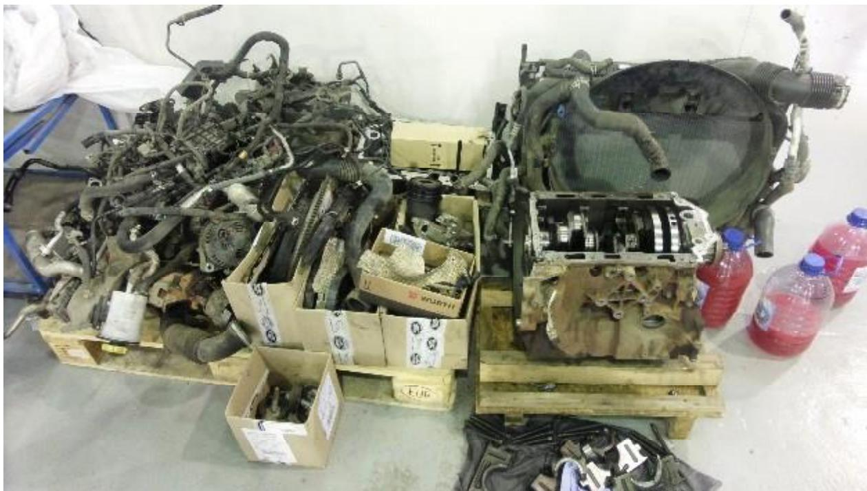
Fig. № 5. dismantled and disassembled engine attachments of the test vehicle
