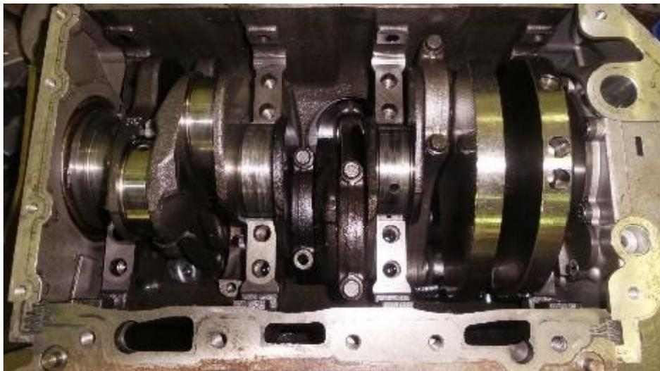
Fig. № 6. disassembled, with removal of the pallet, the test car engine LAND ROVER DISCOVERY 4
