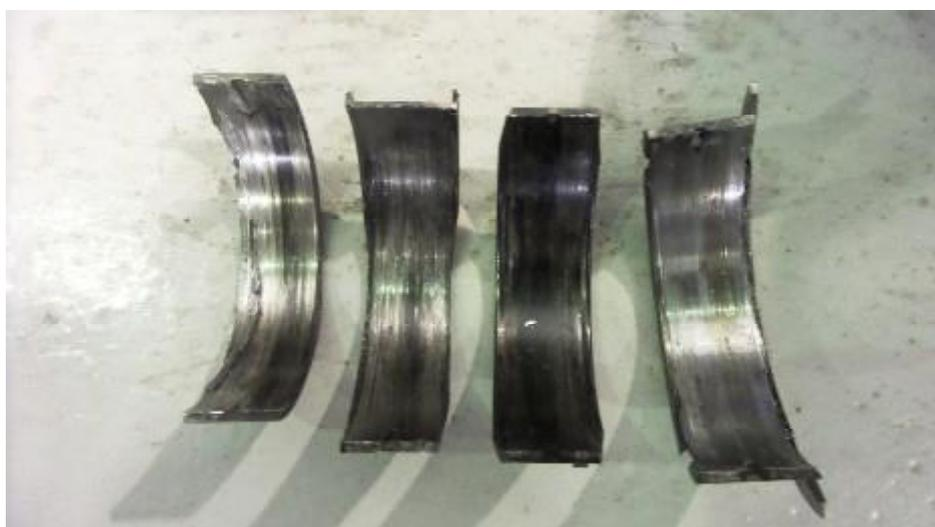
Fig. № 8. Native neck engine inserts the test vehicle LAND ROVER DISCOVERY 4, VIN
