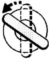
**5. Enter the FOURTH number of the code.** If the fourth number is 1, turn the key to the LOCK position once. Ensure the key is FULLY returned to the centre position.
