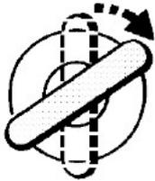
**4. Enter the THIRD number of the code.** If the third number is 12, turn the key to the UNLOCK position twelve times, ensuring that the key is FULLY returned to the centre position
