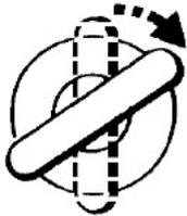
**6.** Finally, turn the key to the unlock position once more. If the code has been entered correctly, a double 'bleep' will sound (a single 'bleep' indicates that the code has
