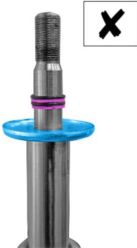
6. Install the lower O-rings and spacers as follows, spacer, O-ring, spacer, O-ring and spacer.
