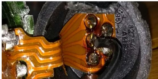
all I have done too fix mine is literally cut back the burnt pcb ribbon neatly ( not on above picture these are just samples. And using a very flexible 12v wire I soldered it to the top of the micro switch connectors and black plug connectors to reestablish a connection and they work fine again. If your switch is this burning causing the fault. Its only a small trigger signal and so a small very flexible 12v wire is all that I used,
