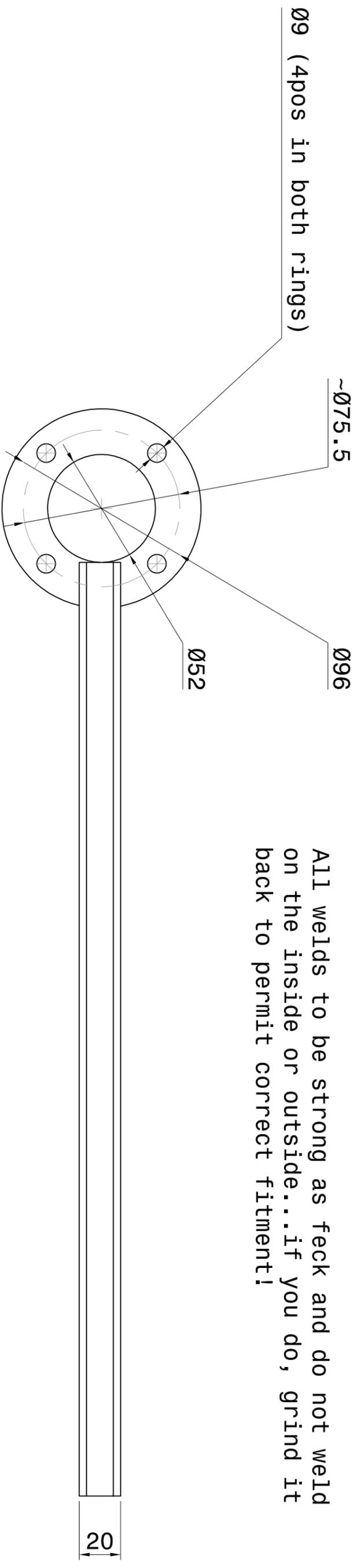
All welds to be strong as feck and do not weld on the inside or outside...if you do, grind it back to permit correct fitment!
