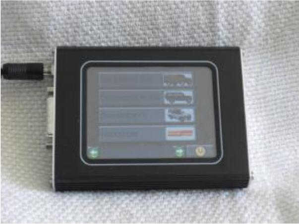
For each vehicle menu there is a submenu with the entire diagnostic modules available for that vehicle.
