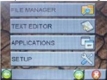
If the NANOCOM has a start up mode other than "NORMAL", then the main menu will be shown only after an application is selected and the Nanocom will then exit the start up parameter.
