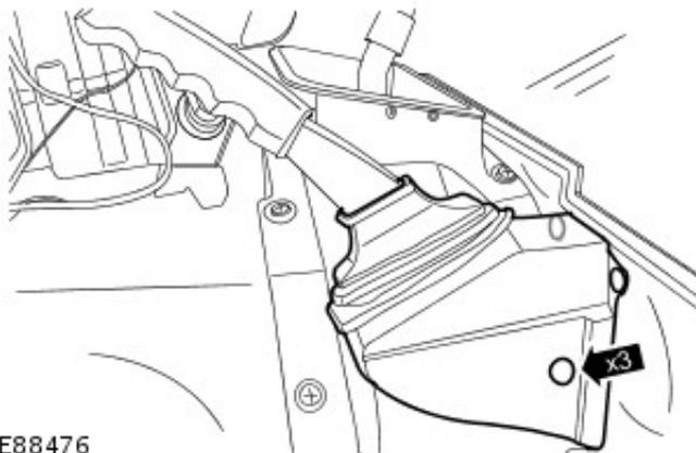
2. Remove the parking brake lever clevis pin.
