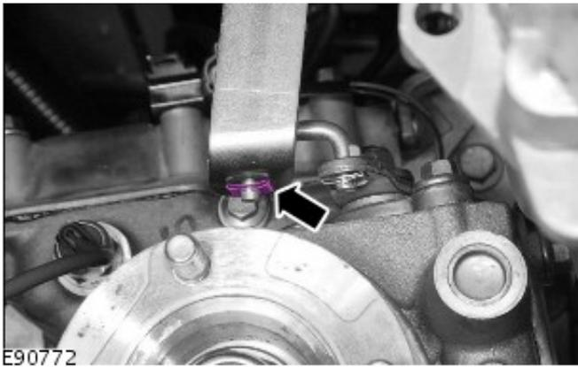
**18.** Remove the differential lock control operating rod.
