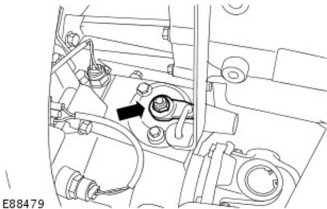
**19.** Release the transmission wiring harness.
