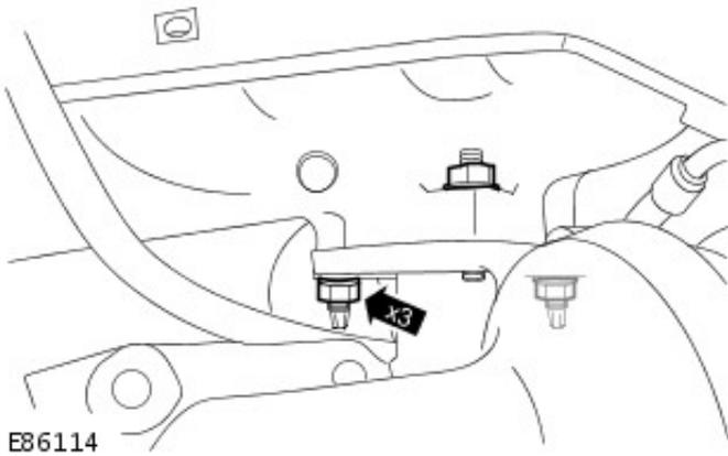
**13.** Remove and discard the 3 turbocharger nuts.
