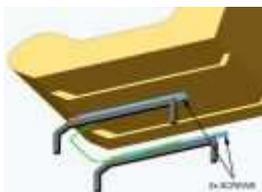
Store the seat somewhere. Now remove the four screws holding the red track to the frame. Gain access to screws by sliding the top tracks to the opposite side. The handle is sprung outwardly against the tracks so it will want to spread them apart, so when you are on the last 2 screws just squeeze the handle free ends together and remove it:
