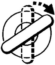
**1. Using the key,** turn the driver's door lock (clockwise) to the LOCK position and hold in this position for at least 5 seconds. Then return the key
