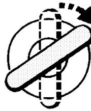
**3. Enter the SECOND digit of the code.** If the second digit is 3, turn the key to the LOCK position 3 times. Remember; the key must be FULLY
