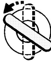
**2. Enter the FIRST digit of the code.** If the first digit is 4, turn the key (anti-clockwise) to the UNLOCK position 4 times. Ensure the key is
