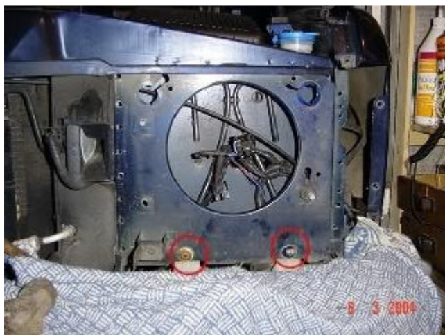
PASSENGER SIDE SHOWN WITH WASHER BOTTLE MOUNTS CIRCLED RED
