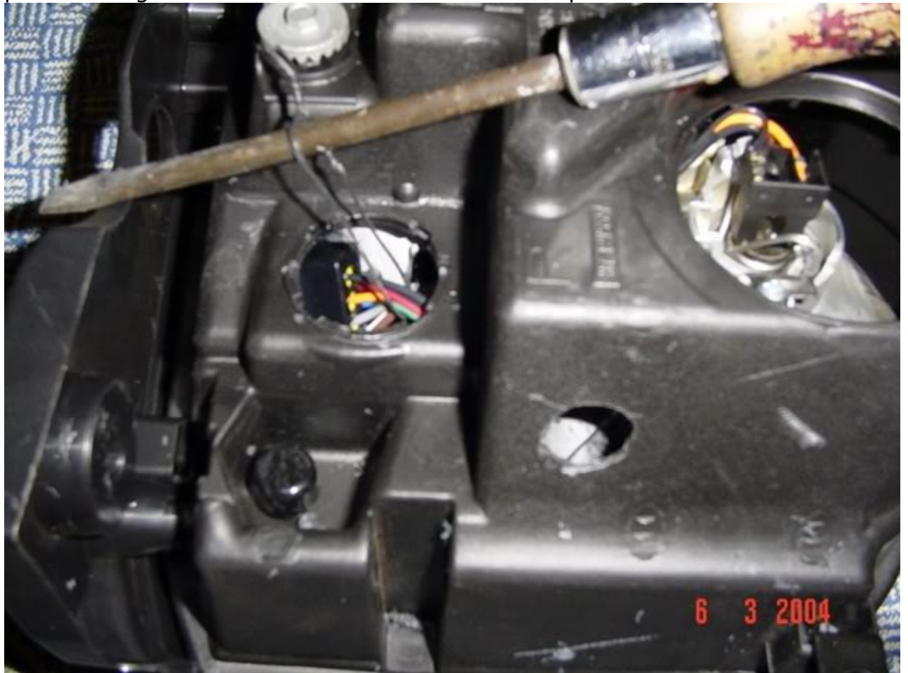
PHOTO SHOWING SOCKET WITH WIRES ATTACHED - TWINE USED TO PULL WIRES CLOSE TO THE HOLE
