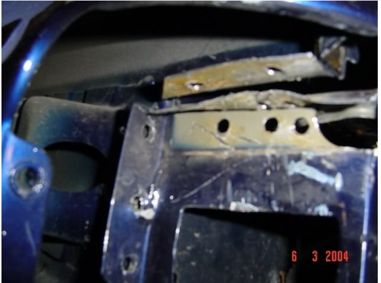
SPOT WELDS AT TRIPLE SEAM BELOW FRONT WING-SHOWING SEAMS FOLDED UPWARD - THIS SEAM MUST BE RE-WELDED OR SECURED
