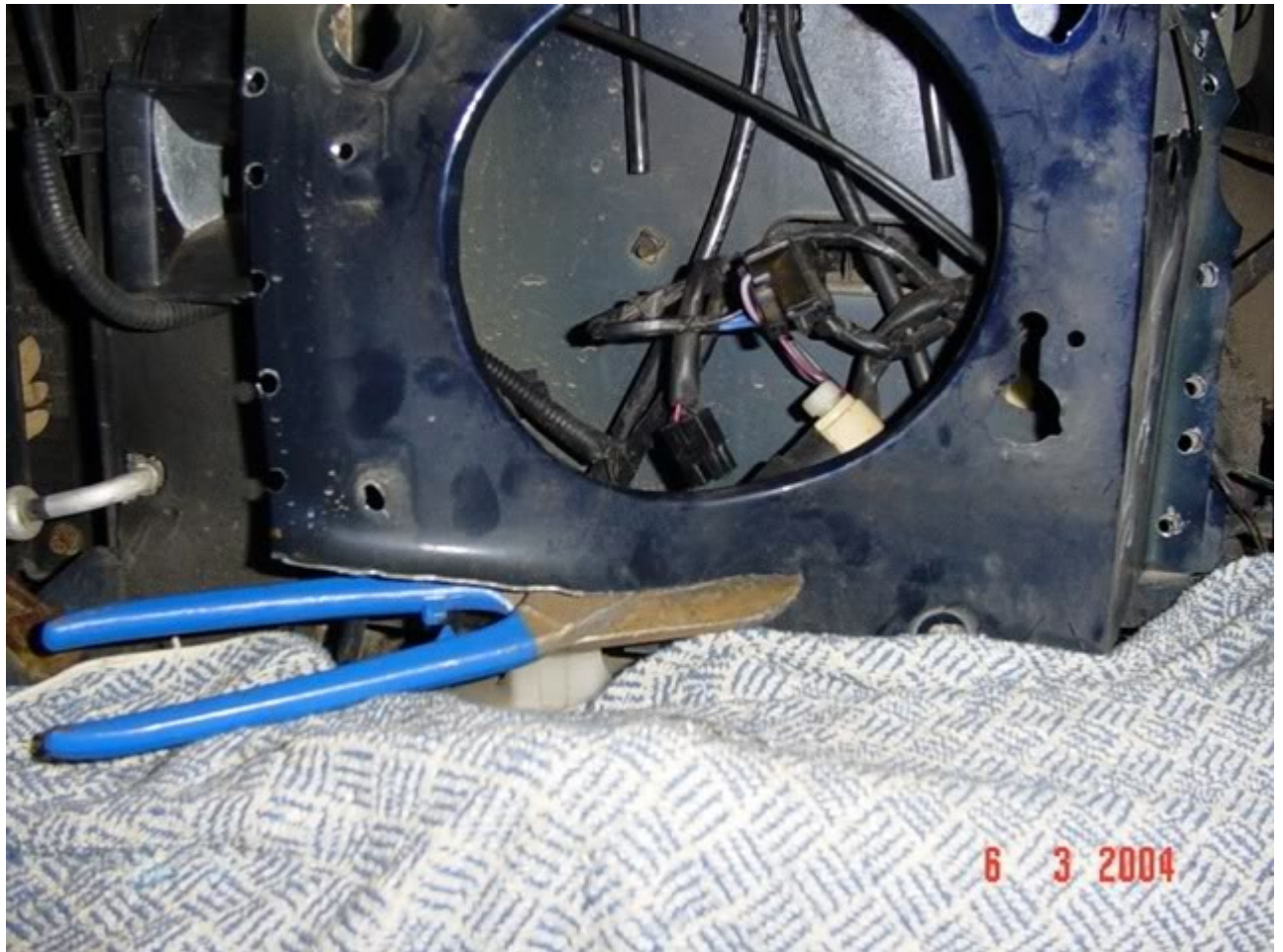
PASSENGER SIDE SHOWN - CUTTING ALONG BASE WITH SNIPS
