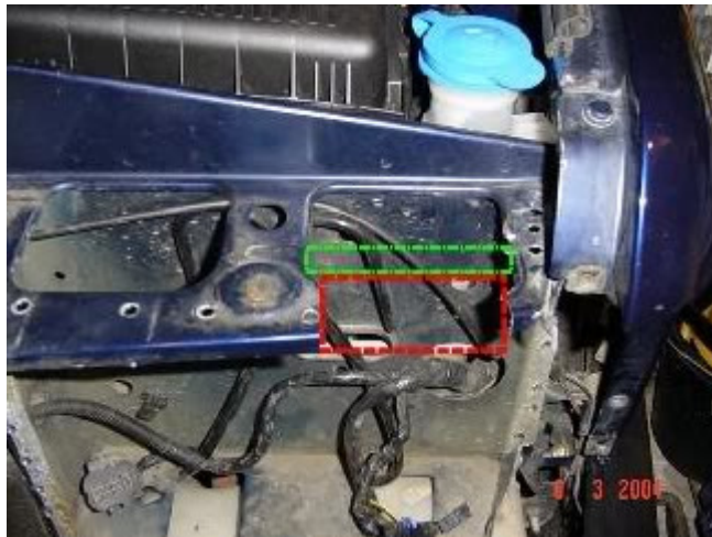
PASSENGER SIDE SHOWN - CUTTING ALONG BASE WITH SNIPS
