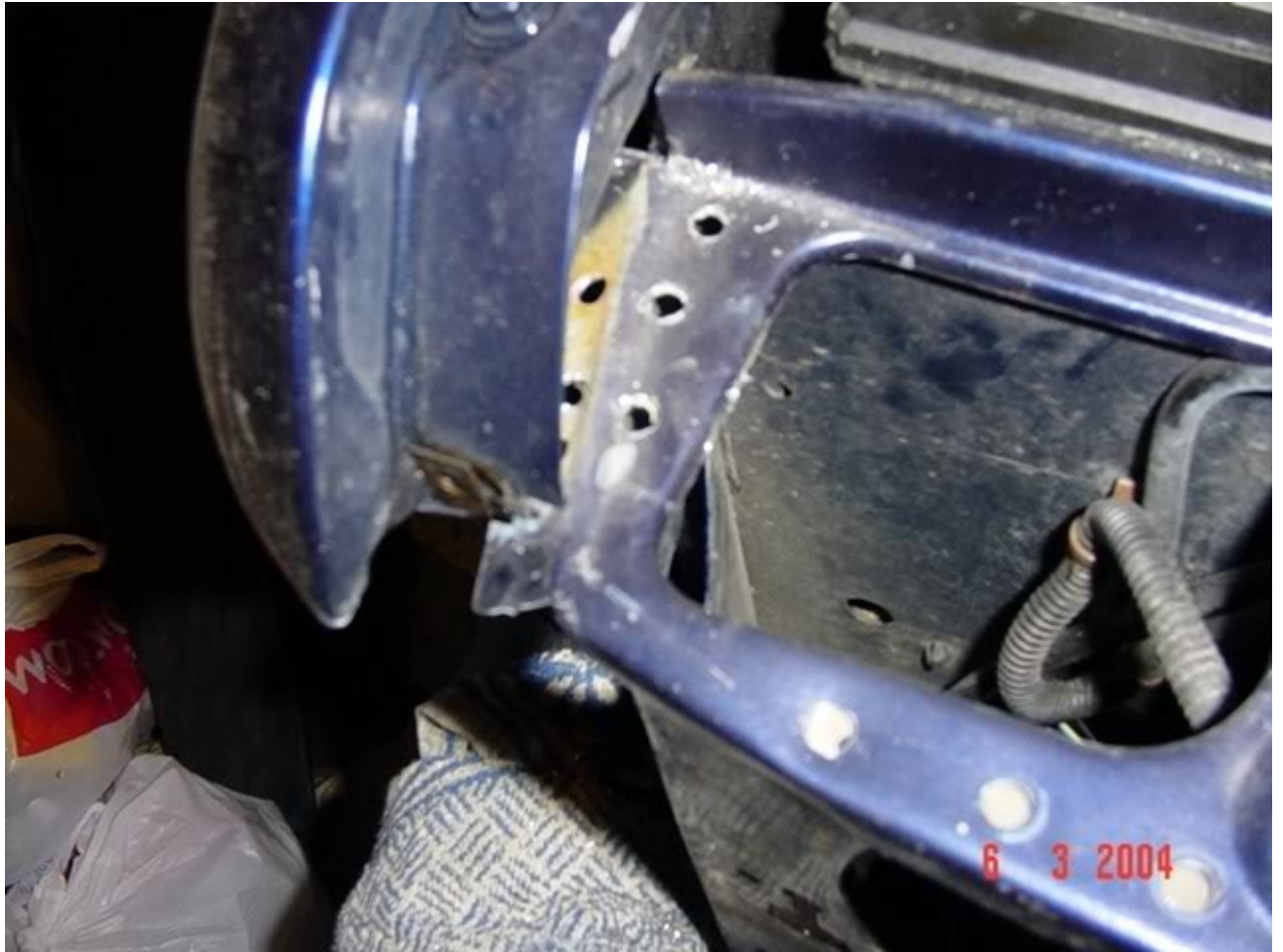
SPOT WELDS AT TRIPLE SEAM BELOW FRONT WING
